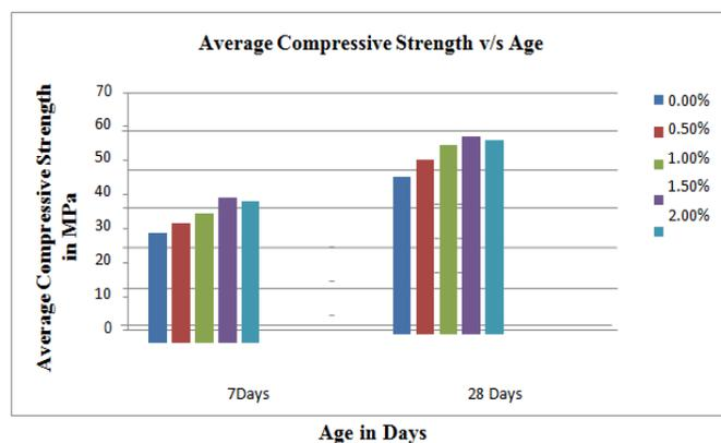
Figure 3: Average Compressive strength of concrete with Cement replaced by micro silica at 7 and 28 days
